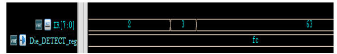
Fig.14 Test data register access to detect number of dies present in SoC
