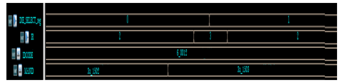
Fig.7 Read access of IDCODE and MAN_ID registers at MTAP level
