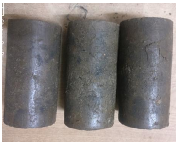
Fig. 7: Failure of 28 days cured sample of an optimum mix
