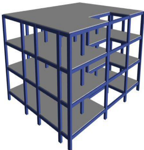
Fig 2a: G+2 RC Structure without Infill
