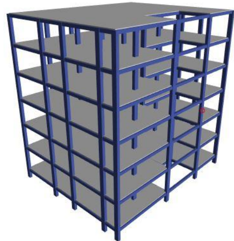
Fig 3a: G+5 RC Structure without Infill
