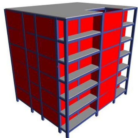
Fig 3b: G+5 RC Structure with Infill
