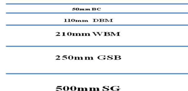
Fig 5.4 Pavement Section showing thickness of various layers for stabilized black cotton soil.
