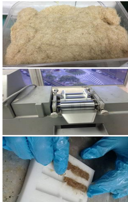
Fig 1 (a) Chopped kenaf fibres (b) Three roll shear milling machine and (c)Mixture of kenaf and epoxy resin is placed in the silicone mould
