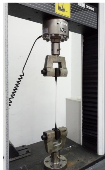
Fig. 3: Specimens under tensile test
