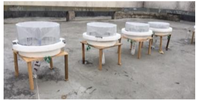
Fig. 3 Solar stills of 15°, 20°, 25°, and 30° condenser plate tilt angle
