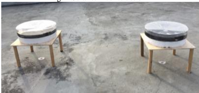
Fig. 2 Solar stills with PVC (left) and PP (right) condenser plates
