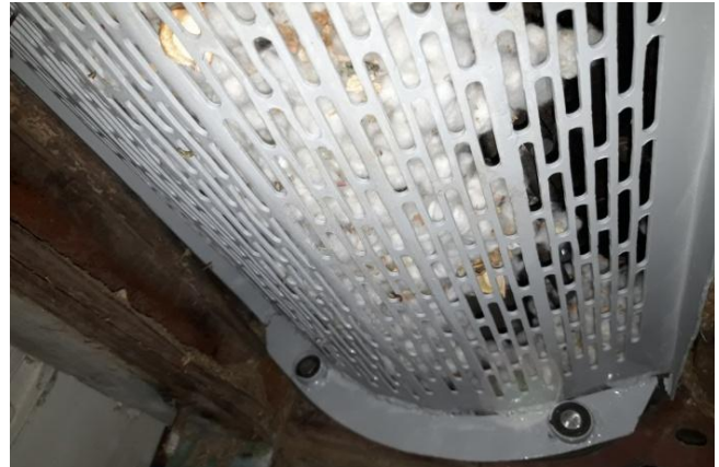
Figure 7. A prototype of a multifaceted grid surface mounted on the UGC cotton ginning unit
