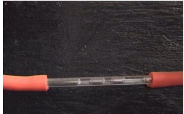
Fig.12. Flow observed in PHP at different Heat Input.
