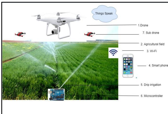
Fig.1: Smart watering equipment
