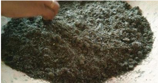
Fig.4 Soil mixed with fiber
