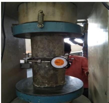
**Fig.1. Testing of wrapped cylinder**
