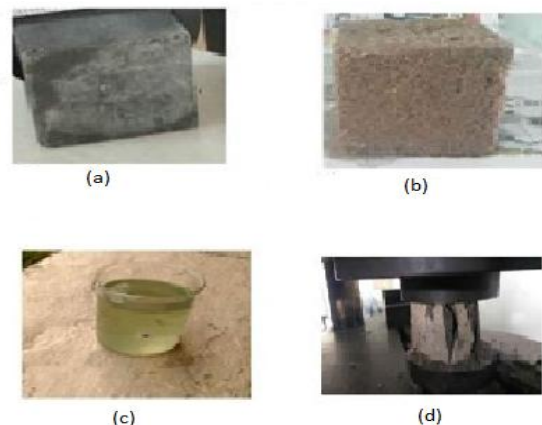
Fig.3: Chloride penetration area in the mortar specimen and testing, (a) Normal cube, (b) Chloride penetration area in mortar specimen, (c) Chloride solution reacted with mortar specimen, (d) Testing of mortar specimen
