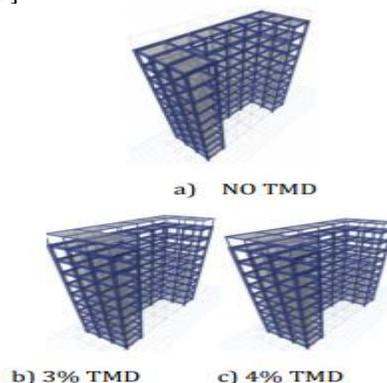
Dislodging, quickening, base shear, story glide are more without the proximity of TMD. By setting TMD, best case scenario of the structures, removing, expanding speed, base shear, story skim are decreased. TMDs are all the more convincing in diminishing vibrations.
