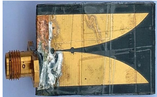
Fig.4(b): Fabricated Double cavity Vivaldi antenna
