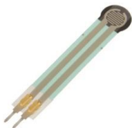
Fig.2 Pressure sensor to obtain the pressure data
