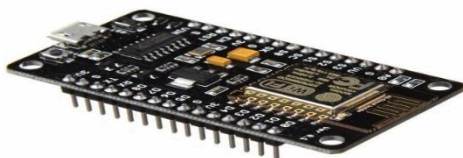
Fig.3 Node MCU with an ESP8266 built-in module
