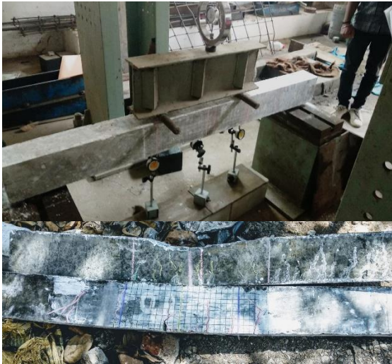
Fig 8. Showing test setup and failure modes of two specimens without and with Nano GGBFS.
