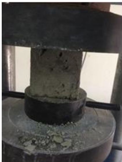
Fig. 4: Concrete cube applied with load
