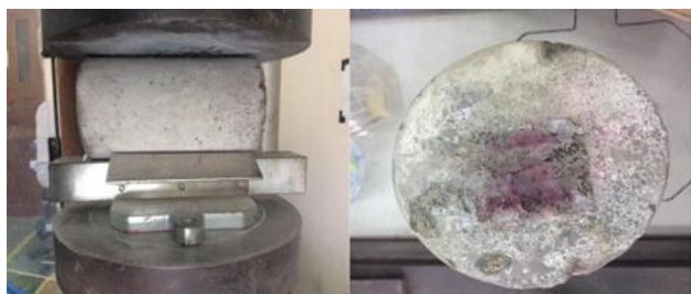
Fig. 5: Concrete cylinder applied with load
