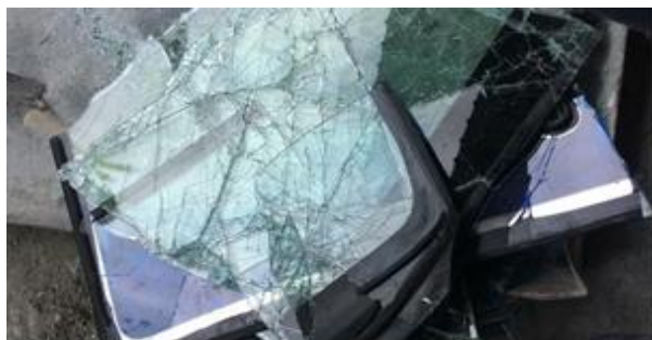
Fig. 1: PVB laminated windshield glass
