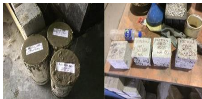
Fig. 3: Concrete sample of (a) cylinder and (b) cubes
