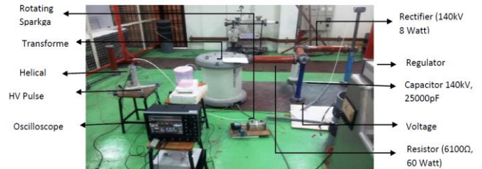
Fig. 2. Experimental setup used for static PEF treatment
