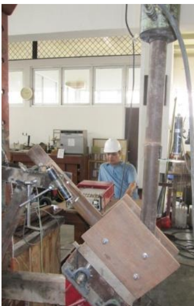
Fig. 3. Test set-up for connection system models with quasi-static loading
