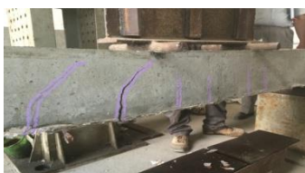
Fig. 1: Experimental test setup for SCC composite beam
