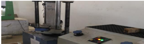
Fig. -7 - Universal Testing Machine With Specimen
