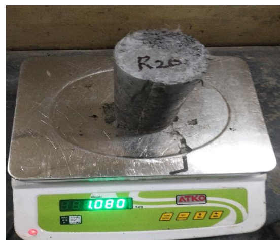
Fig.2 ECC Cylindrical specimen with 20% of RHA & 2% of polypropylene fibre
