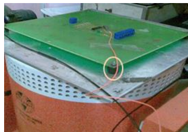
Figure 4 PCB assembly mounted on rubber spacers
