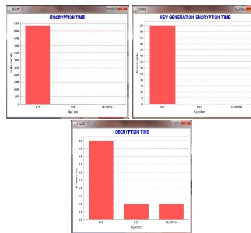
Fig.4 Uploaded data is encrypted using AES,DES and blowfish and cipher text is shown along with time taken for encryption and decryption.
