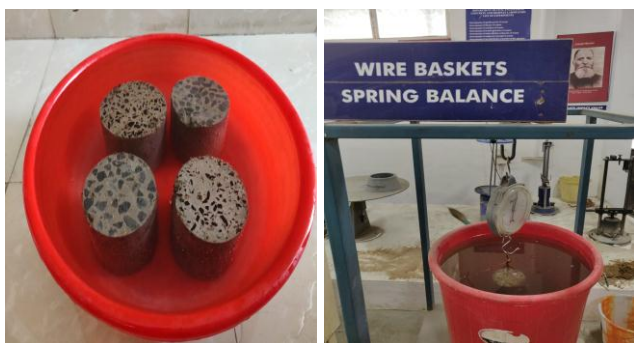
Fig. 4 Specimen under VPV test
