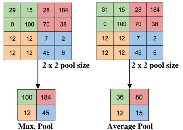
Pooling is done to reduce the spatial dimensions of the input data to the next convolutional layer. The transformation is either performed by taking the maximum value or the average value from the window. It is also called down sampling. Max pooling is preferred due to its better performance. Max pooling is followed for first few layers and average pooling is followed for the last layer.
