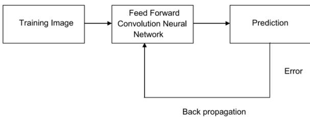
In this system, the feed forward CNN used on the training image. If the predicted output is not correct, back propagation is used.
