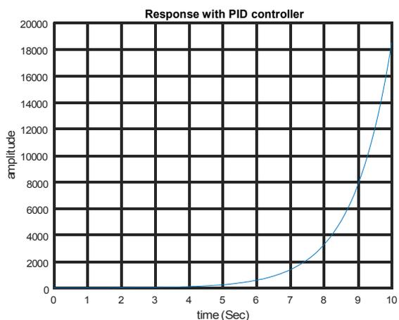
Figure 6. PID Output Response of Manipulator
