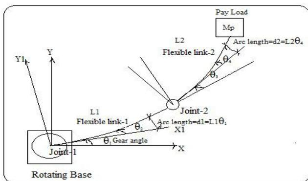
Figure 2. Gear, Deflection angles & Link Position
