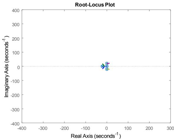
Figure 3. Root Locus Graph of Serial link Stability
