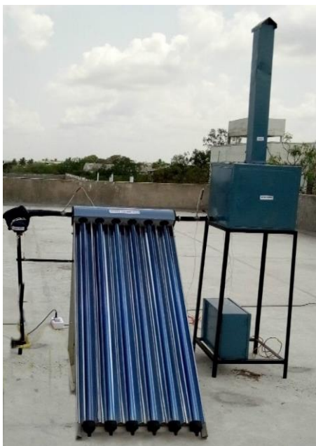
Fig. 2.1: Photograph of Evacuated Tube Collector Based Solar Dryer
