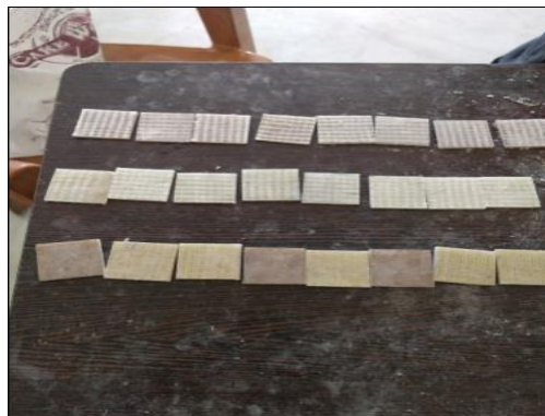
Figure 6: Water Absorption tested samples
