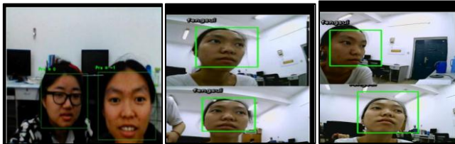
Figure No. 3 (a) Multi-Face recognition: Two people facing the camera can be acknowledged (b) Left: Harr-like outcomes Right: LBP outcome with deflection slant.
