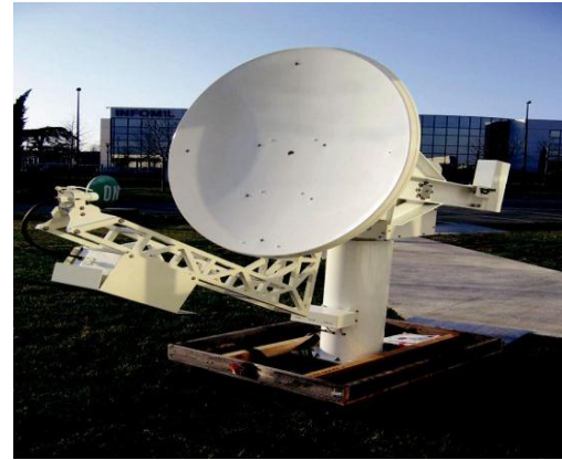
Fig.1 : CNES dual frequency single polarization outdoor Earth station
