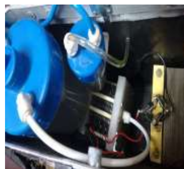
Fig. 5 Assembled HHO water gas flame torch and its components
