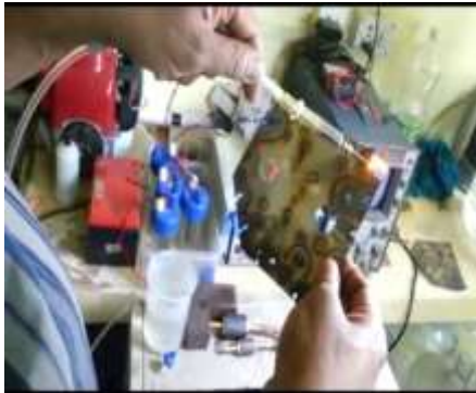
Fig. 6(a) Cutting of Iron using HHO Flame Torch
