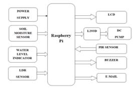
The Smart garden enclosure framework keeps up in total activity of the porch nursery and all the sensor devices and DC siphon will be related with Raspberry Pi. The Raspberry Pi module constantly gets data from sensors and picks the with pre chosen conditions. In case the condition satisfies, by then controller send web notice to customer and hold up to get commitment from customer with a scope of time interval.
