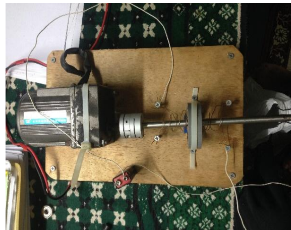
Fig. 4: A laboratory scale EMC torque transducer.
