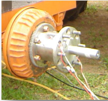
Fig. 1: Strain gauges embedded torque transducer [7]
