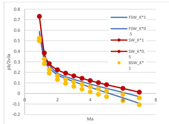
**Fig. 6: Influence of wing swept angle due bending stiffness reduction**
