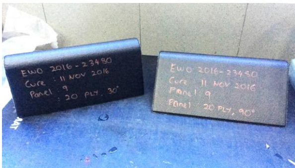
Fig. 3: Curved specimens after being extracted from their mold tools.
