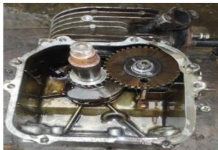
Fig. 1: Modified air-cooled, 4-cycle, vertical, single cylinder gasoline engine
