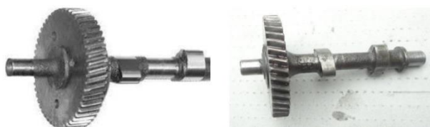
Fig. 2: General camshaft with egg shape cam and modified cam shaft with eye shape cam
