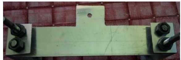
Fig. 12: Jig to hold the inner mirror
