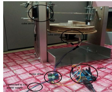
Fig. 11: Arduino to servo connection
