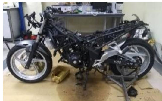
Fig. 4: Fuel engine mounted on the chassis
