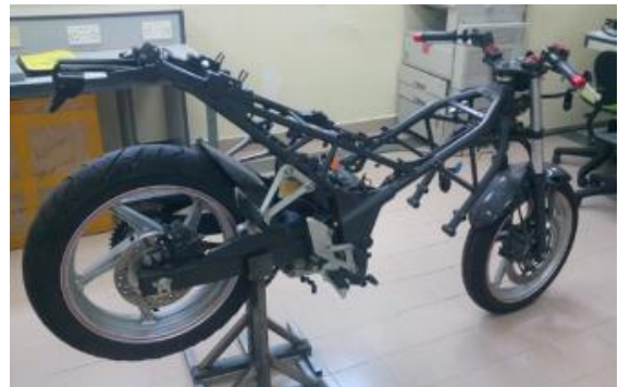
Fig. 3: After removing fuel tank, fuel engine
