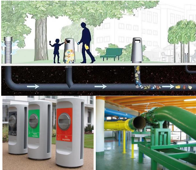
Figure 9 Pneumatic system flow (Source: Amaravati Concept Handbook)
