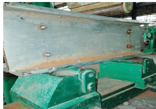
Fig. 2: Point bending test arrangement
