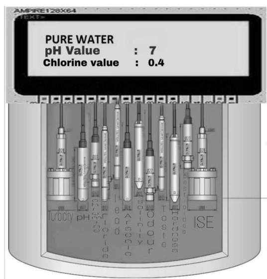
Fig. 4: Prototype of system & how sensors immersed in water tank and displays result
