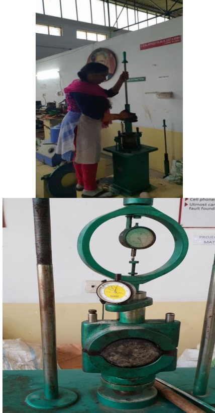
Fig. 1 Marshall stability test Sample testing
