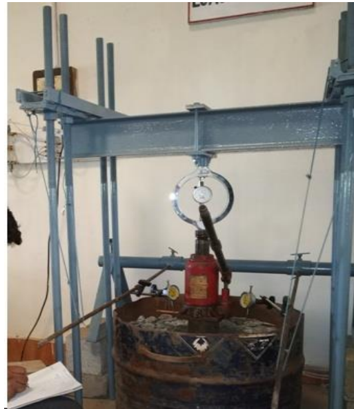
Fig. 5 Experimental Cyclic Plate Load Set For Finding Load – Settlement.
