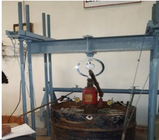
Fig. 5: Experimental Cyclic Plate Load Set For Finding Load - Settlement
