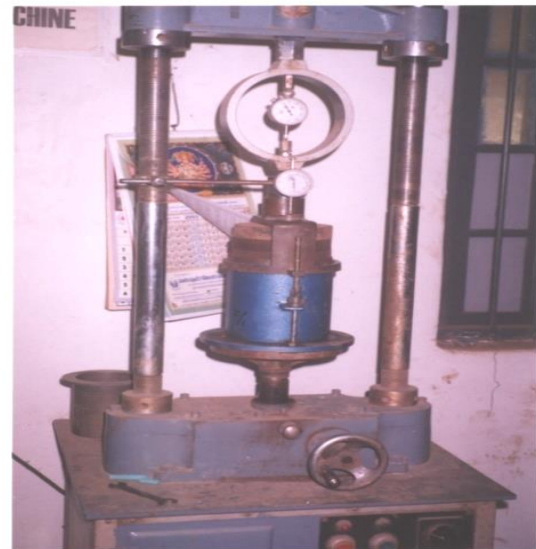
Fig. 4: California Bearing Ratio Test Apparatus
