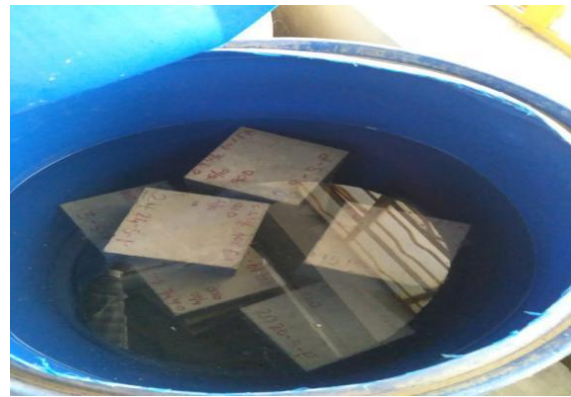
Figure 2: Cubes Exposed to NaCl solution
