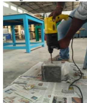
Figure 3: Cubes during and after drilling
