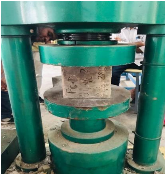
Figure 5: Compressive Strength of Cubes
