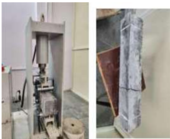
Figure 6: Flexural strength of PUMICE lightweight aggregate concrete prism along its failure
