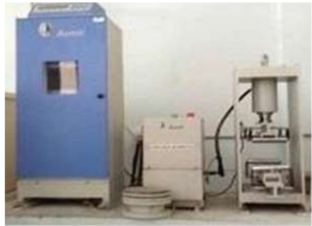
Figure 7: Split tensile strength test using Automatic Compression Testing Machine
