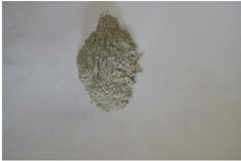
Fig. 5: Collected concrete powder after drilling
