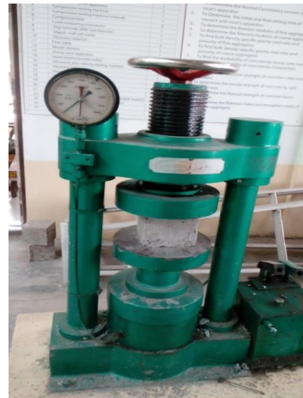
Fig. 1: Compressive testing of cubes
