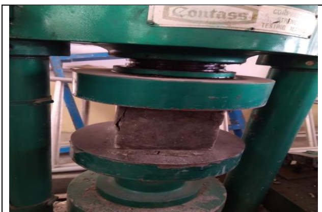
Fig. 1: Compressive Testing Machine (CTM)
